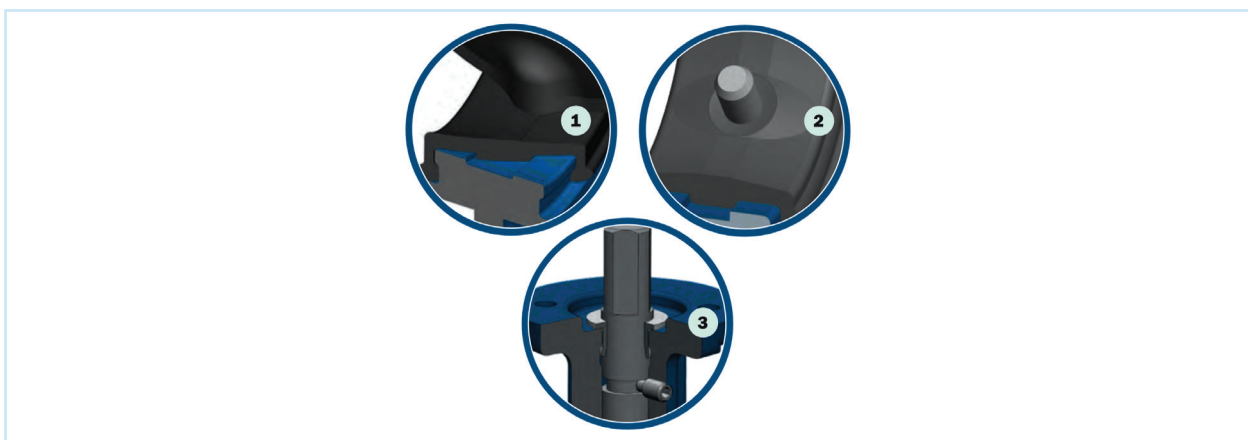
FIG. 11 - 3-STAGE SEALING SYSTEM
